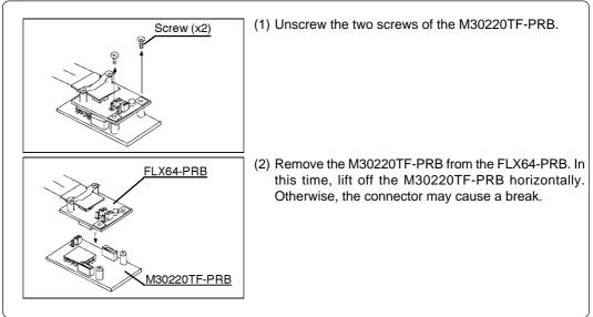
Figure 3.4 Removing pod probe M30220TF-PRB
